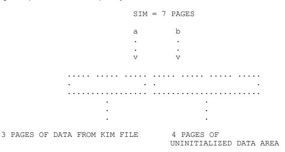
If the space available on the system tracks only allows the data through "a" to be written to disk, SYSGEN will issue an error message and terminate execution. If, however, the system tracks could hold the data through "b" then SYSGEN will execute normally. In either case the user's code in BOOT and SIM must keep track of the load addresses and the number of tracks/sectors to load.
