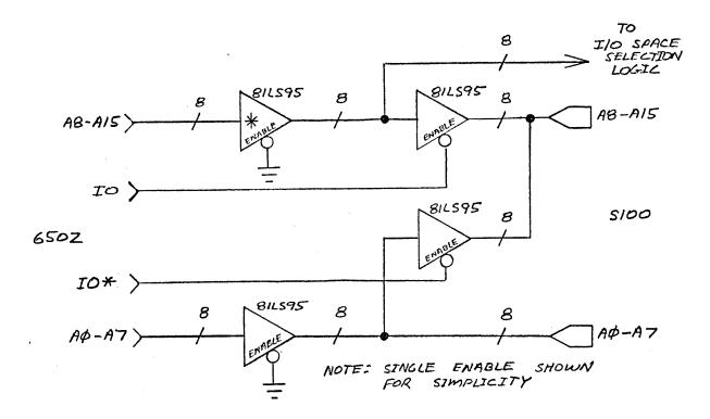
Figure 2-3. 6502 to IEEE Standard 696 Address Bus Interface
