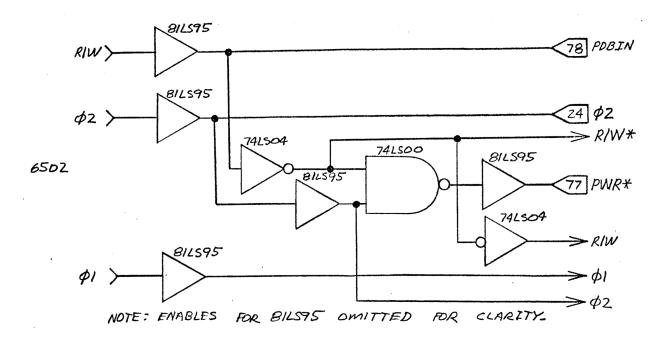
Figure 4-1. Primary Control Signal Outputs
