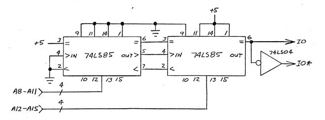
Figure 4-3. IO Decode Logic (For E0xx)
