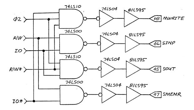
Figure 4-2. Secondary Control Signal Outputs
