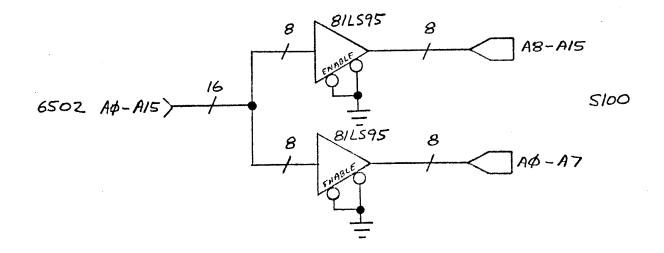
Figure 2-1. Simple 6502 to IEEE Standard 696 Address Bus Interface
