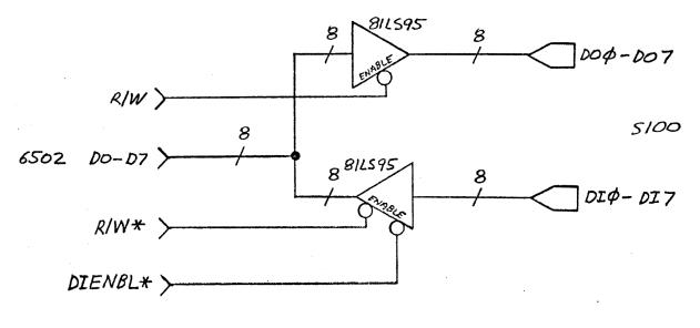
Figure 3-2. 6502 to IEEE Standard 696 Data Bus Interface
