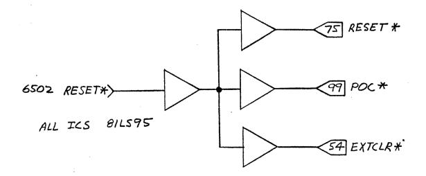
Figure 4-4. IEEE Standard 696 Reset Logic
