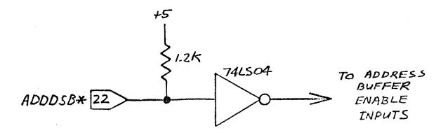
Figure 2-2. Typical Address DMA Modification
